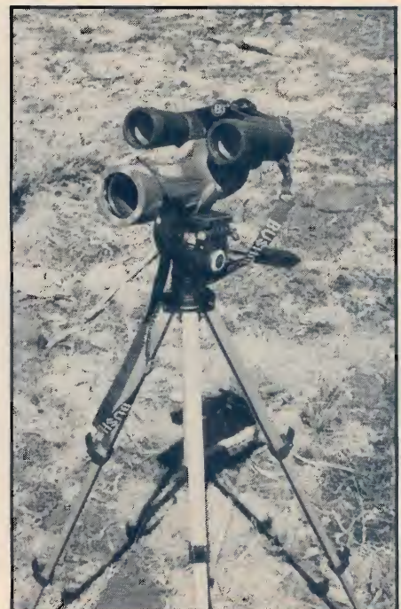
Here is one way to keep both a spotting scope and binoculars stable.
